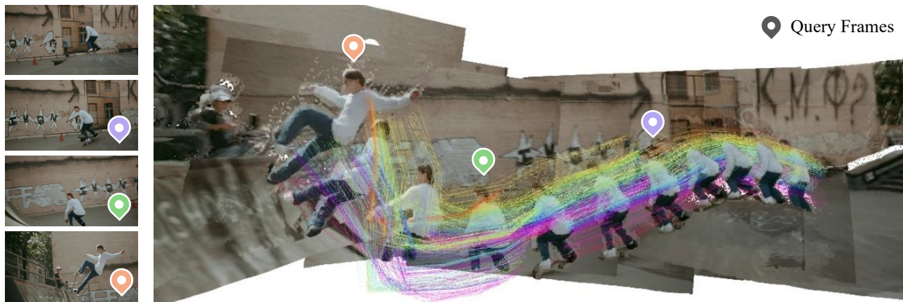
Figure 1. 4RC (pronounced “ARC”) enables unified and complete 4D Reconstruction via Conditional querying from monocular videos in a single feed-forward pass. It jointly recovers camera poses and dense per-frame geometry, while supporting flexible querying of dense 3D motion from arbitrary source frames to any target timestamp.
